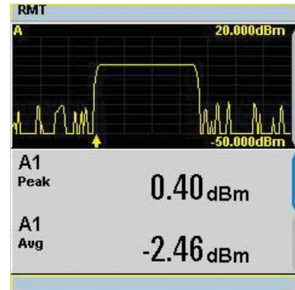
Figure 12. Effects of VBW on a power meter measurements of a radar with fast rising pulse edge.
